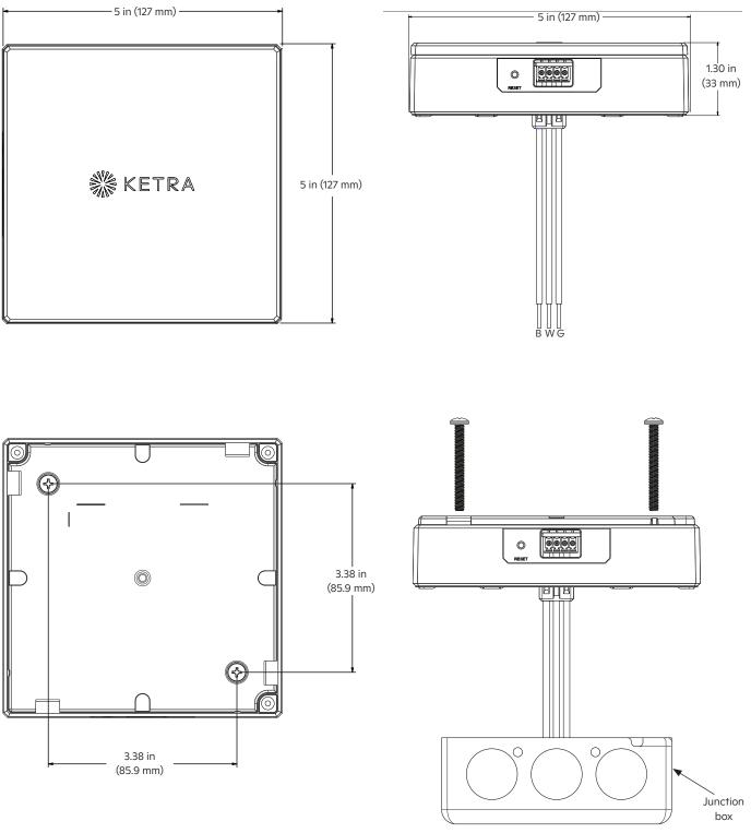
Mounts to standard 4 in x 4 in (101 mm x 101 mm) junction box. Junction box not included.
