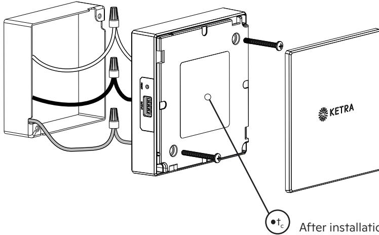
After installation, measure the temperature in this location to verify controller is operating within spec (158 °F [78 °C] max).
