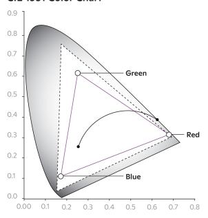
Ketra's G2 high output linear accent can easily be commissioned into Lutron HomeWorks or Athena systems. The product can reproduce any color point within the triangle shaped gamut indicated in the chart to the left. With Ketra's Color Lock tool, the color point is maintained to an accuracy of one-step MacAdam Ellipse over the lifetime of the product and across operating temperature range.
